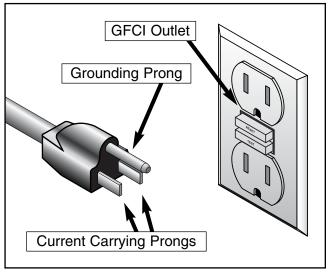
**Figure 1.** NEMA 5-15 plug and GFCI outlet.
